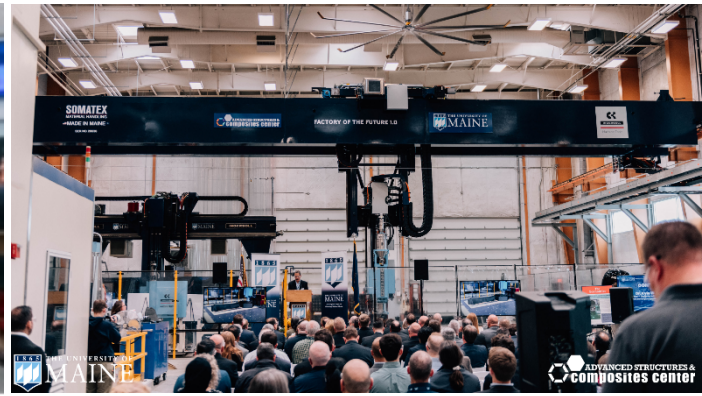
Figure SEQ Figure \* ARABIC 2 Factory of the Future 1.0 dedicated in April 2024, includes two large printers and five end-effectors capable of up to 500lbs/hr deposition rate, continuous tape layup, 5 axis machining, and robotic arm manipulation. The larger printer has a build volume of 96ft long x 32 ft wide x 18 ft high and the smaller one 60ft long x 22ft wide x 10 ft high. They are connected to a HPC and a suite of sensors.
