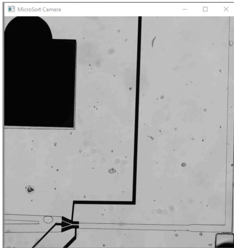
Figure Microscopic view of feeder, sorting and waste channels, along with the electrodes
