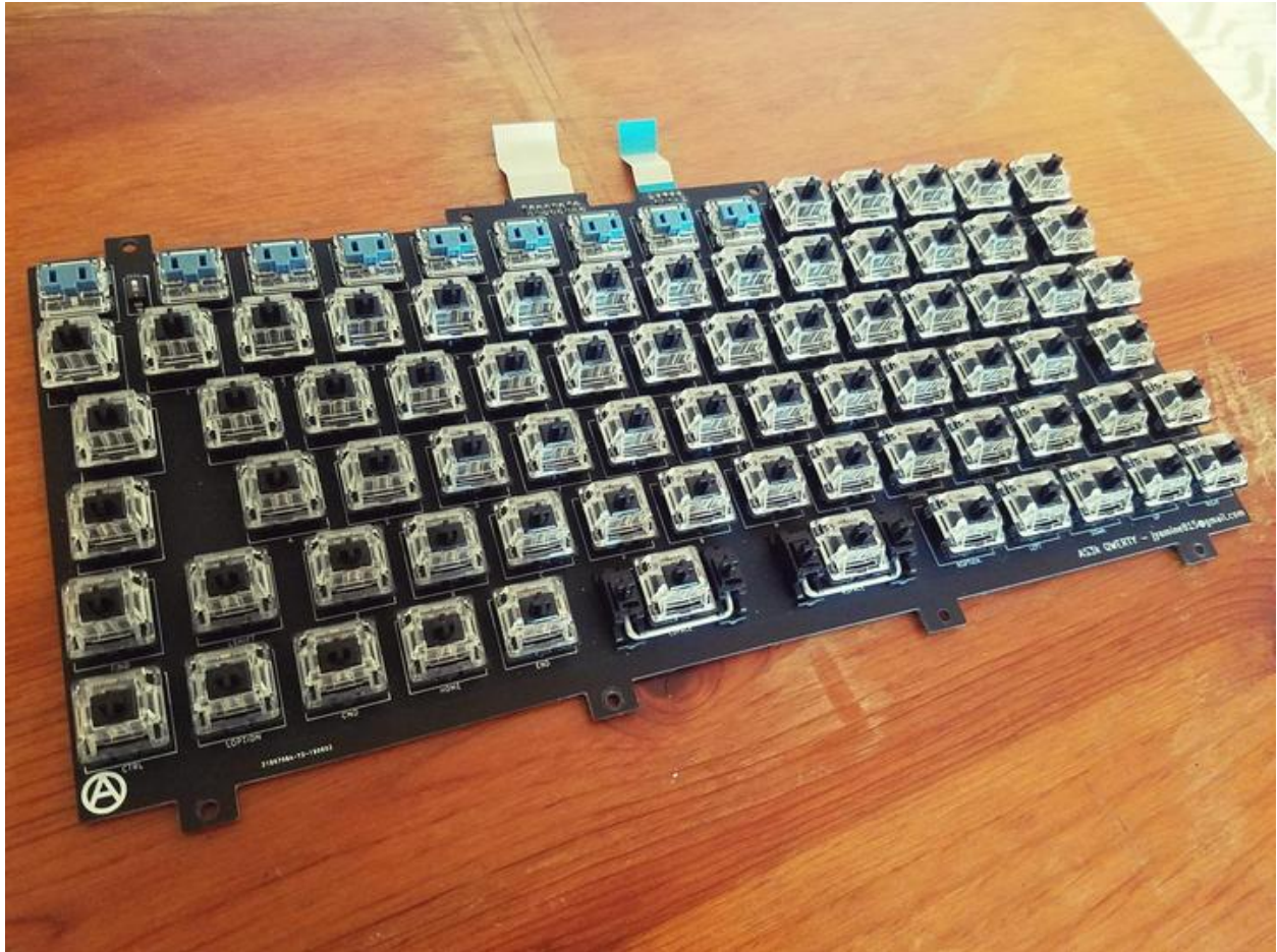
Example of stabilizers on custom board.
