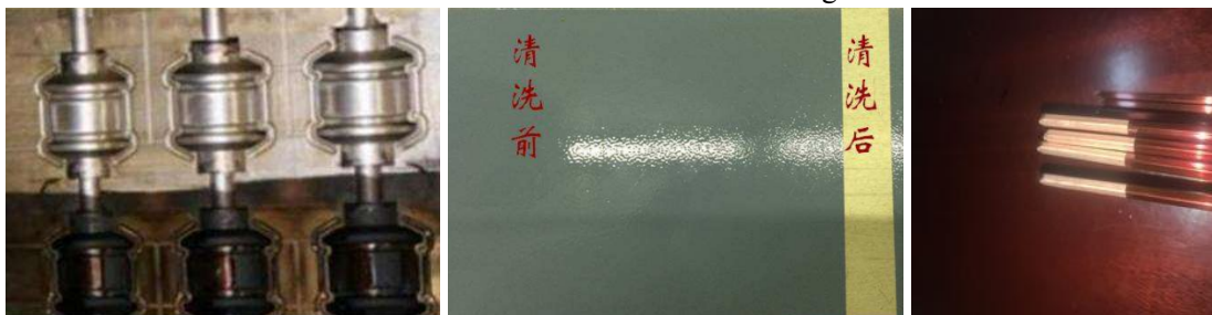
C Laser cleaning of oil and paint stains
