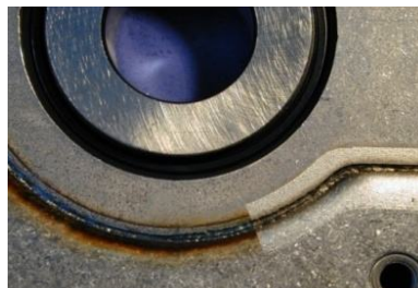
b Metal surface oxide laser cleaning
