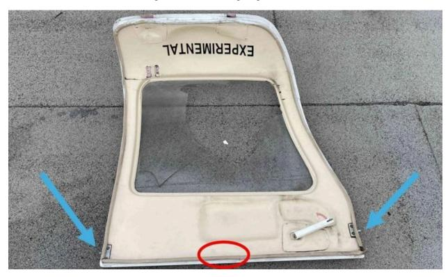
Investigators found the left cabin door of the Van's Aircraft RV-10 that crashed January 2 on the roof of the same warehouse that the airplane struck while attempting an emergency landing at Fullerton Municipal Airport. Blue arrows point to the primary door latches, and the area where a secondary latch should have been installed is circled in red. NTSB image.
