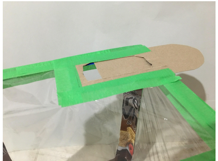
12. Install the sliding ventilation gate.
