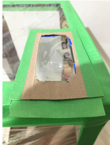
10. Tape the pocket to a corner on the roof. Use two sides of the frame to provide support for the ventilation gate holder.
