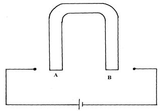
Complete the diagram showing the windings on the magnetic material so as to produce polarities
