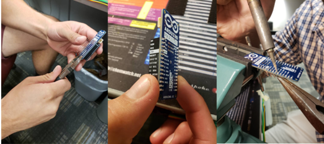
Figure S2: Removing Factory Pins from Arduino MKR ZERO
