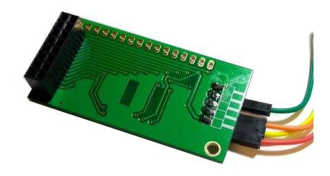
10. We will now plug the LCD into the i2c Backpack. It is extremely important that all pins are aligned properly (*shifting them one way or another will damage the LCD and/or the i2c!*) do not force them.
