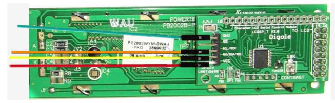
12. Prepare the pieces of wire (each ~4" long) by stripping end of insulation (if not already stripped) and tinning with solder (but not too much or it will not go in the hole).
