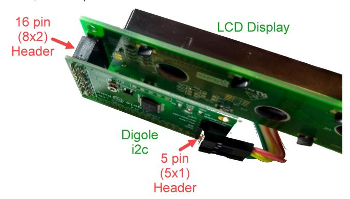
11. Plug the four color-coded M-F jumper cables onto connectors on i2c board.
