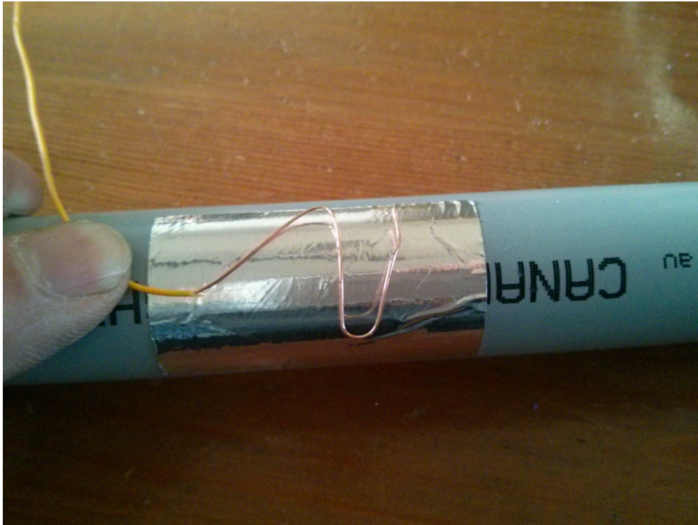
Photo 6 - ZigZag wire to increase contact area.
