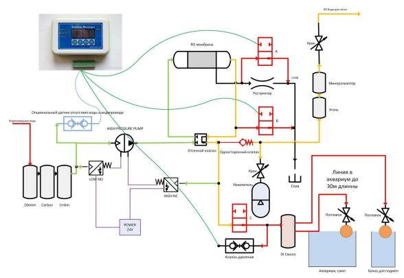
The pressure sensor in the line of the float may be in two different versions. Low and high sensitivity. low sensitivity sensor comes as standard and allows you to use longer lines for connecting the float. Connecting low sensitivity of the sensor is carried through, the cut of water supply line to the float. To connect the sensor of high sensitivity or water presence sensor in the water removal is required with the optional tee.
