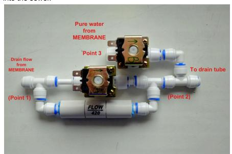
Now we have to install the valve C. This valve is pure water. Its task is to supply water on a schedule in our aquarium. For these valves is put only controls the pressure sensor. Further already provides the water to the resin flask and further into the sump.
