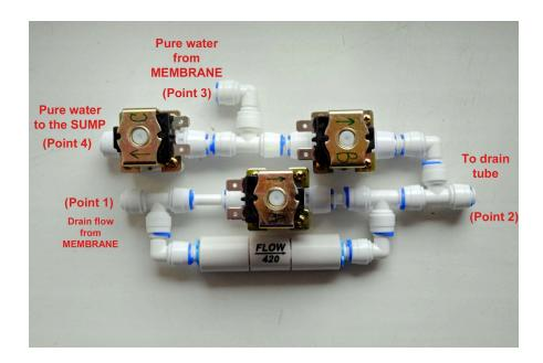
Carefully install all this stuff in osmosis, cut the tube, move, if you want four-way valve closer to the membrane.
