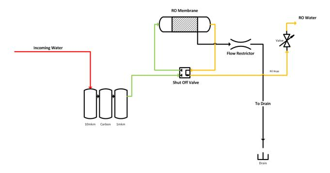
Driving osmosis installation without the pump type Atoll 560 after modification. Red shows the changes being made. Points - tee-fittings.
