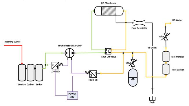
Driving osmosis installation with a pump type Atoll 560 after modification. Red shows the changes being made. Points - tee-fittings.
