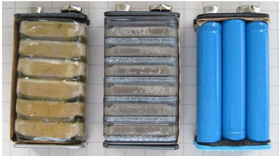
Figure 11. 1.5 V batteries combined to form 9 V battery
