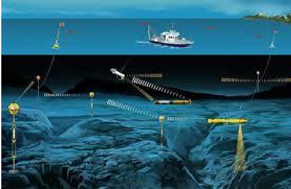
Figure 19. shows water vehicles that use light to communicate with each other and send data between them.
