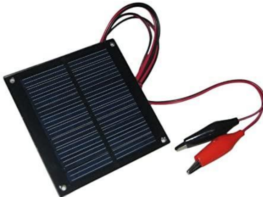
Figure 13. Solar Panel as a Photodetector
