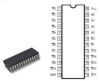
This IC has **4 input** pins (A, B, C, D), **16 output** pins (0-15), **2 enable** pins (G1, G2), and **2 power** pins (Vcc, GND). Output and enable pins are active low.
