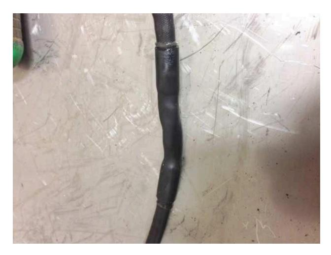
So after the wires have been spliced together, heat shrunk and the sheathing patched you can insert the sensor back into the housing, reinsert the retaining clip and screws and you should be ready to put your Saab 900 Crankshaft Position Sensor back in the car for that satisfying crank, crank, vroom-vroom noise you so desperately want to hear.
