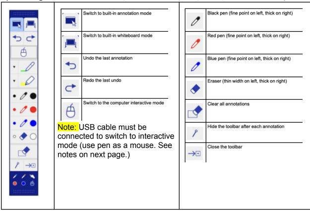
How to: Use the Epson Pen like a mouse to interact with a computer display (and write on the screen).
