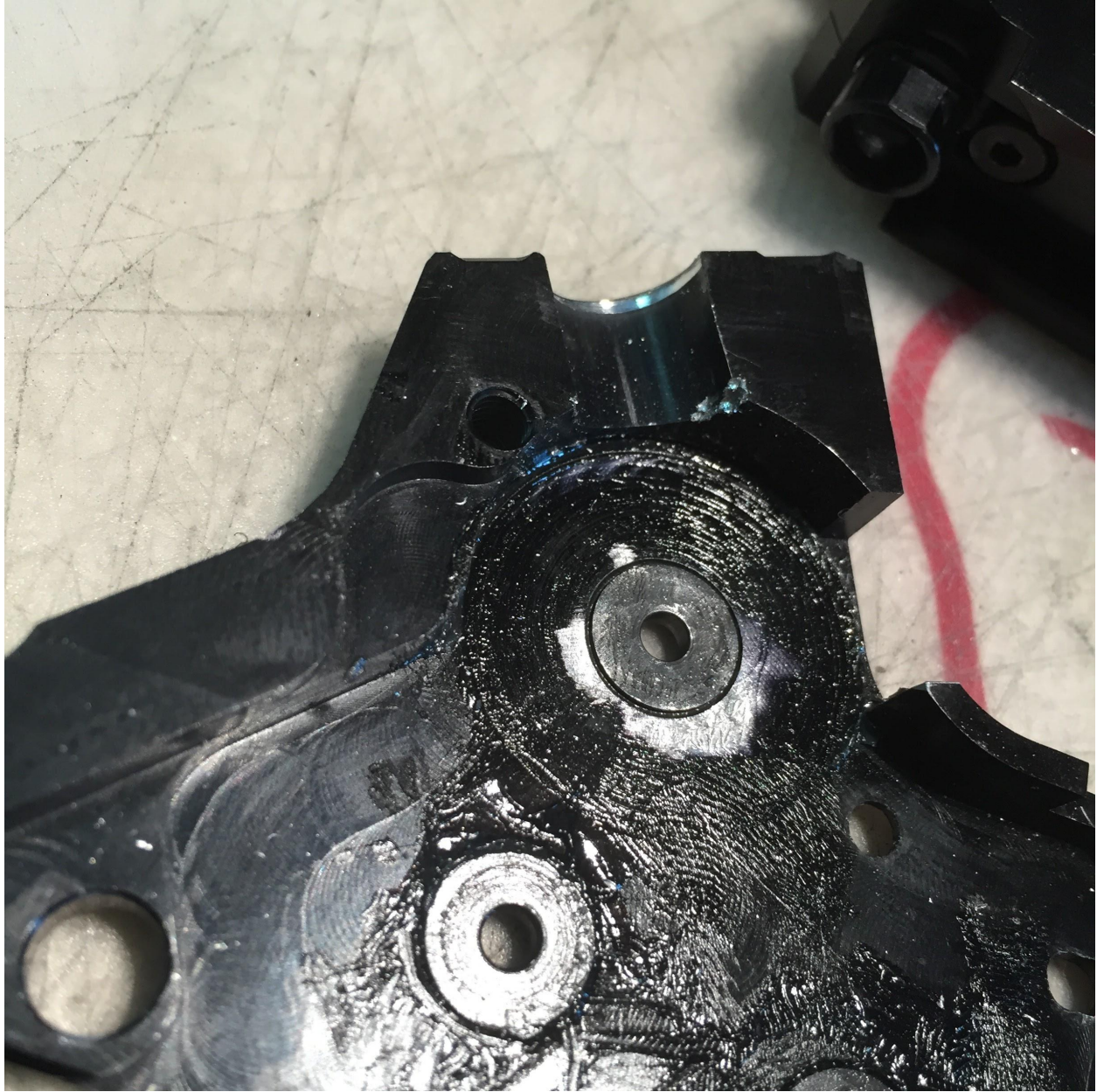
Example of how the lower half of the shell fits in the receiver loosely allowing it to move when screws and pins are put in place:
