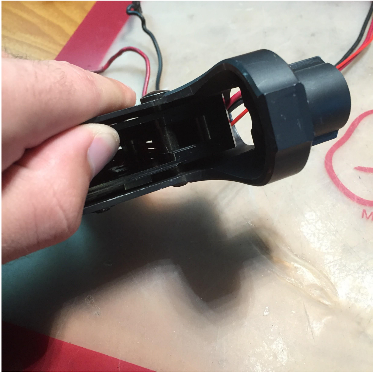
Natural fitment of the lower shell without any pins or screws in at all:
