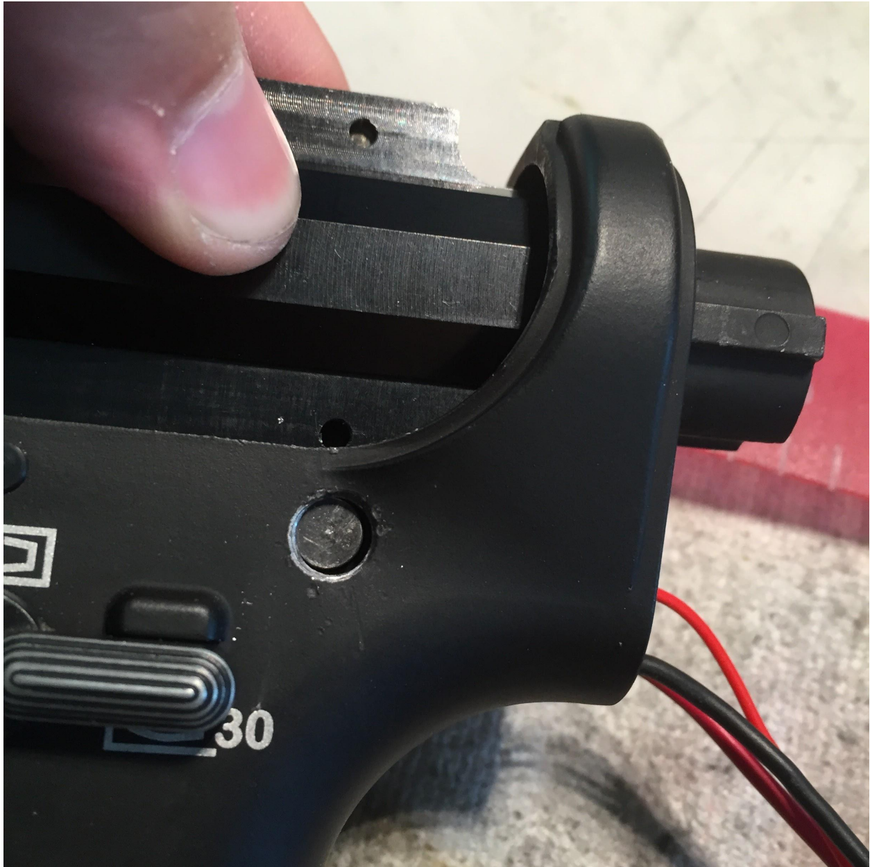
The motor grip pulling down the shell even more, worsening the fitment and alignment of the shell in the body:
