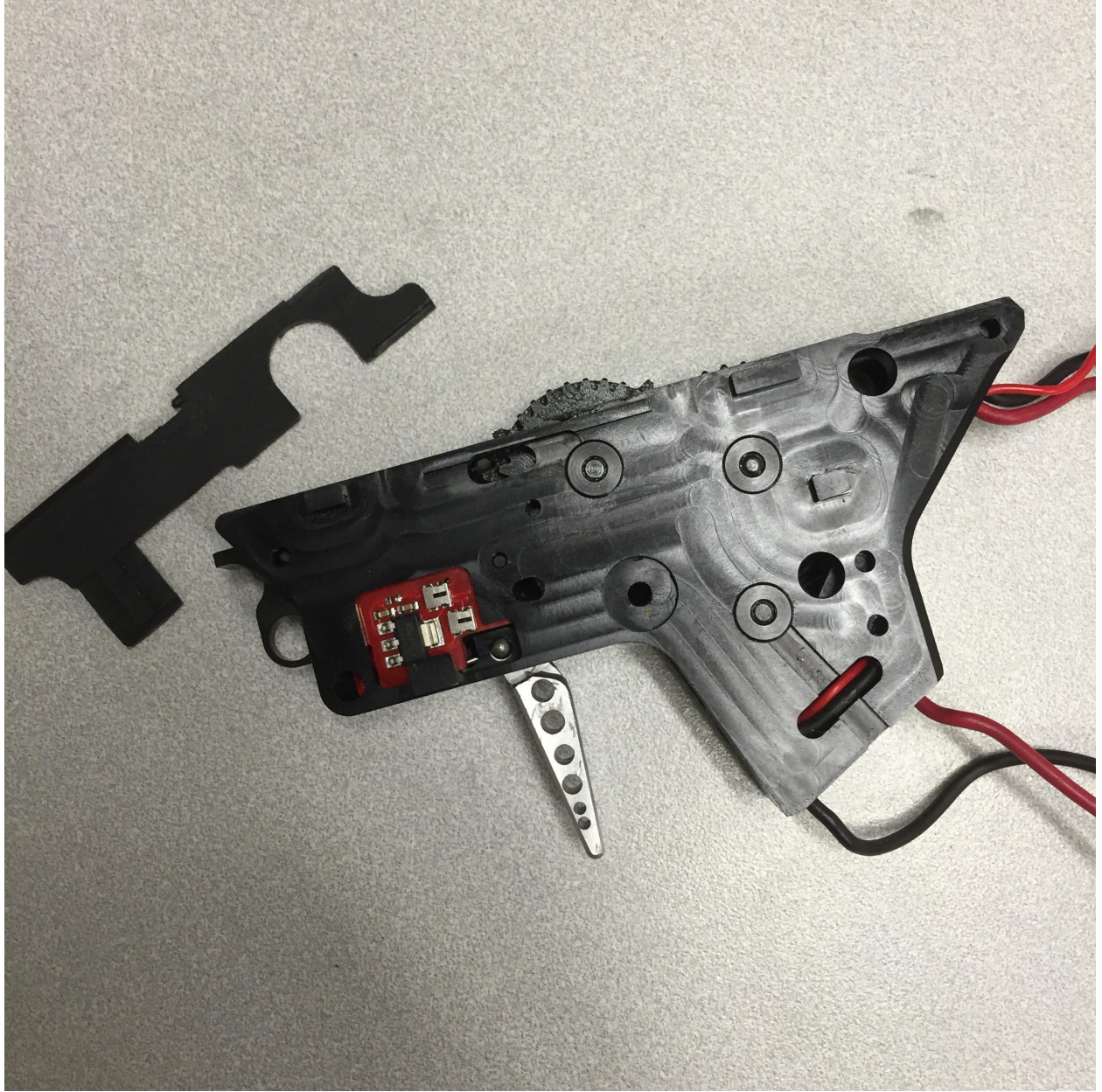
Rail spacing issue resolved with thicker tappets wrapped in electrical tape:
