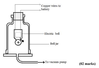
The electric bell is a vibrating source. When there is air in the ball jar the sound of an electric bell is heard to the surroundings (02 marks)
