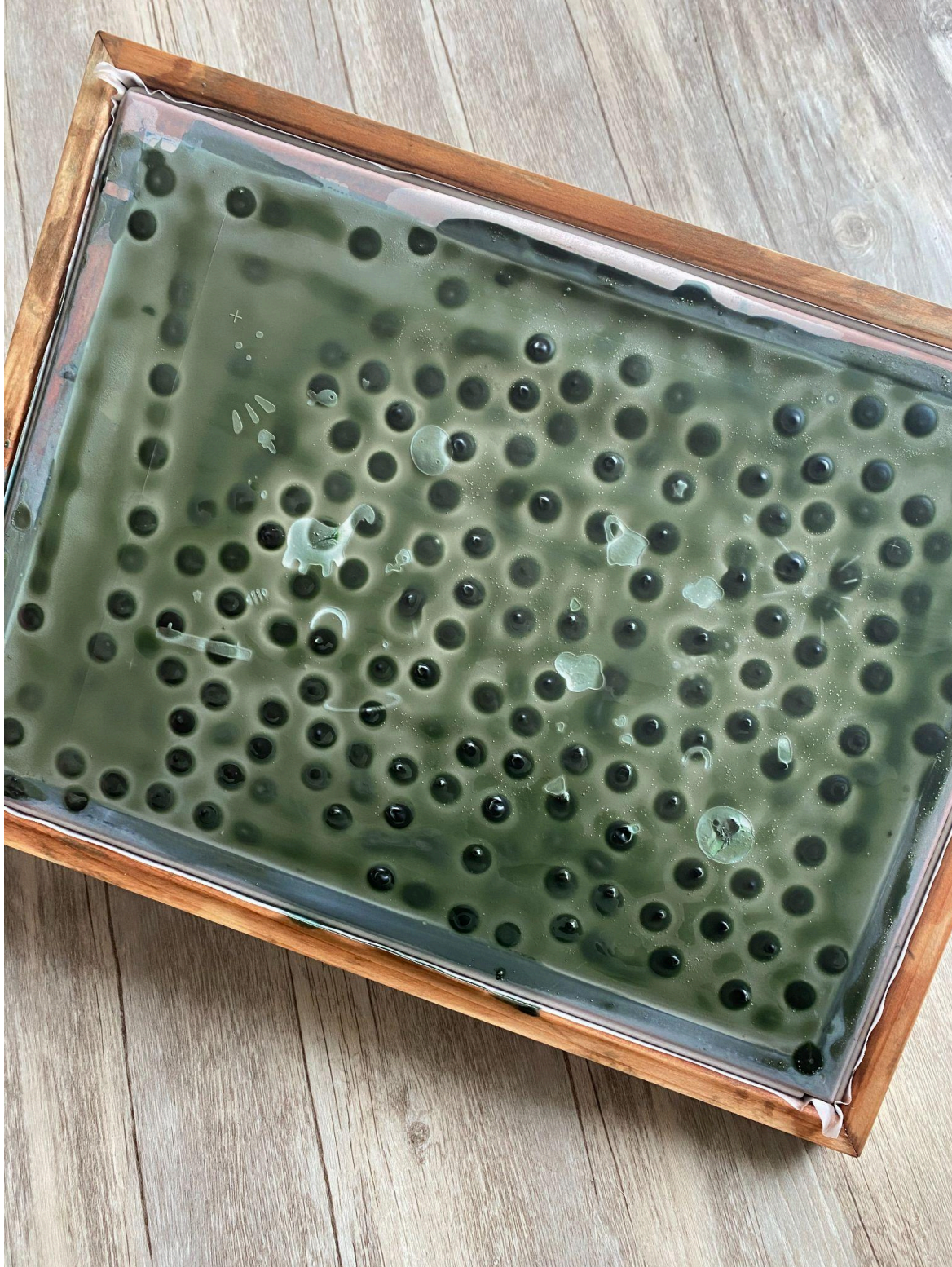
Fig 2. Emulsion coating was way too thick, resulting in drip marks making an uneven surface that was impossible to evenly expose
