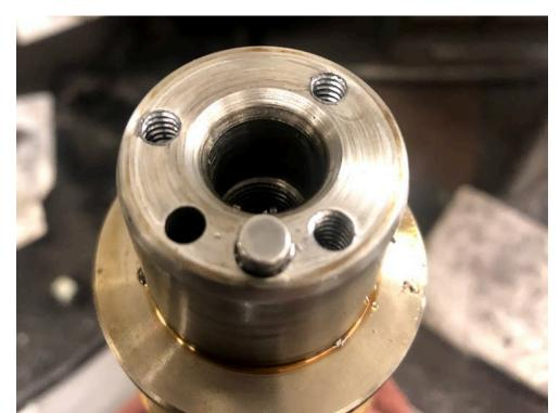
With these ports tapped you can now set the plugs to block off the oil feed! I used 10-64 set screws sealed with Permatex high temp thread sealant.
