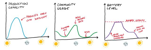
Note that the community usage will be limited by the production capacity of energy by the solartainer. The battery level will be equal to the difference between production and usage at any point in time. Any production that is not used and cannot be stored in the battery is lost.
