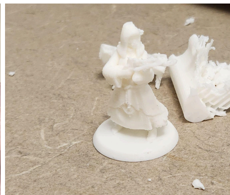
(Don't print with pointy ends pointed down!)
