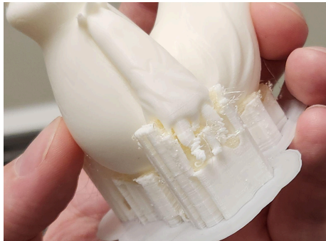
(Don't print with pointy ends pointed down!)
