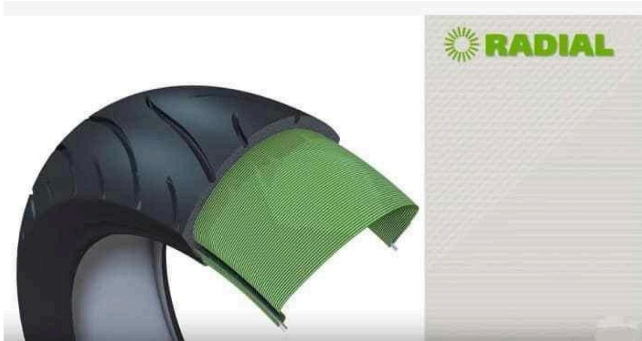
With the radial, you're not stuck compromising the tread rigidity versus sidewall flexibility like you are on a bias ply, which again, has that uniform construction.
