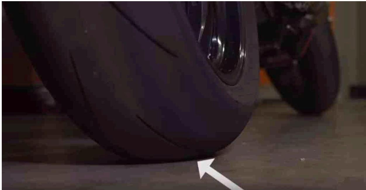
On the other hand, if the pressure is too high you're going to have a small contact patch and a really hard tire, which means less traction and a really rough ride.
