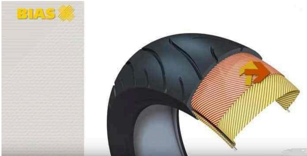
Occasionally an additional layer or two of fabric will be laid just on the tread portion to strengthen that section, but the fabric is still at a diagonal and in general the construction of both the tread and the sidewall are similar so they have similar thicknesses and flex properties.
