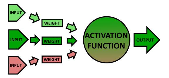
Figure 1: A perceptron. Its likelihood to activate changes depending on the weights (what importance is given to each input) and activation function (how much positive input is needed to activate it). When these are automatically modified, the perceptron 'learns' like a human neuron.
