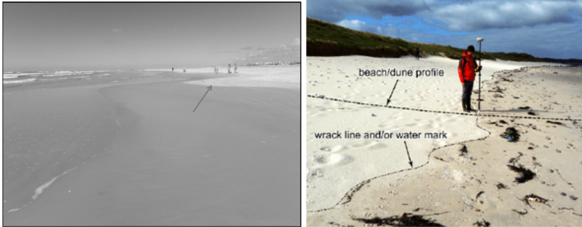
Figure 2: The wet/dry sediment line used as an indicator of the shoreline for GPS mapping (left image indicated by arrow, right image indicated by dotted line) (Suanez et al., 2015).
