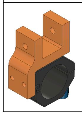
This adapter allows the claw to be mounted parallel to the sub. This allows for the gripper to be mounted lengthwise on the robot.
