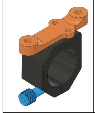
Keep it simple. To the left we attempted to adapt the newton subsea gripper mount to the 80/20 extrusion. However this would compromise the strength of the adapter as it consisted of both injection molded components (the stock gripper clamp) and weaker PLA printed plastic.
