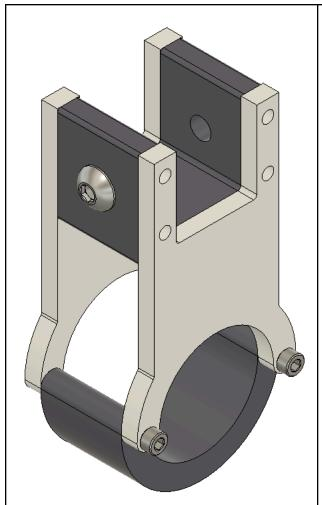
Moved to a combination of 3d printed and delrin cut parts for the holder. The gripper is mounted parallel to the lengthwise bars to manipulate objects right in front of the sub.
