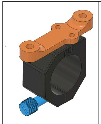
Initially tried a hybrid between the mounts. Here we have the stock newton subsea gripper from blue robotics. This adapter allowed the gripper to be mounted perpendicular to the lengthwise mounting bars.
