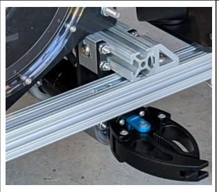
One thing about the final iteration of this design was that the 3d printed pieces (additively manufactured) did not have enough tolerance. This meant that the piece was difficult to mount and even more difficult to work with. In the future, we would add more tolerance to 3d printed parts.
