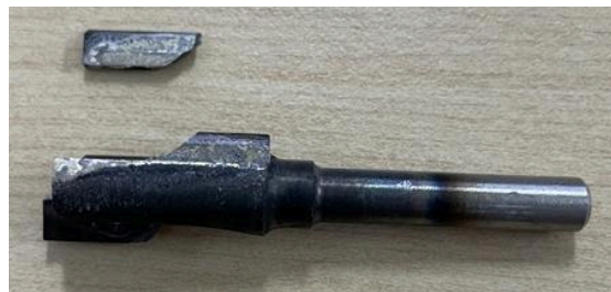
Example of failed hammer test – carbide detached
