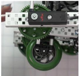
The Rotation Sensor allows Striker's arm to move to the same desired location consistently, eliminating errors caused by other factors. The sensor's absolute value ensures that the desired position is reached every single time, regardless of the starting position of the arm.
