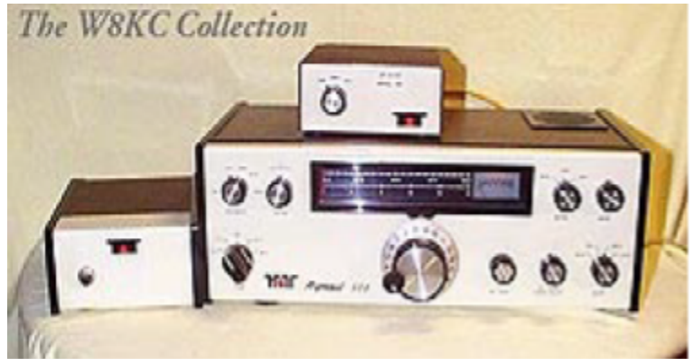
Front view of the Ten-Tec Argonaut 509. The physical appearance of the 505 and 509 models is almost identical. Matching accessories: On top of the radio is the Model 208 CW filter. At the left is the Model 210 power supply (1 A regulated). [Courtesy of the Virtual Ten*Tec Museum.]
