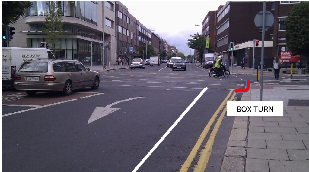
Fig 19 - Outbound lane at Northumberland Road, note there is plenty of space for cycle track and cyclist Box Turn area
