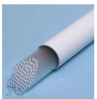
Using a different capillary tube for each sample (careful not to mix them!) transfer a small drop of each solution listed below to the pencil origin line as shown in Figure 1. Apply the six spots evenly along the origin line, but leave a 3 cm margin from each edge of the paper. After applying each solution place the capillary tube back in the sample bottle and not on the table top!! With a pencil, identify each spot by writing on the paper directly beneath the spot.
