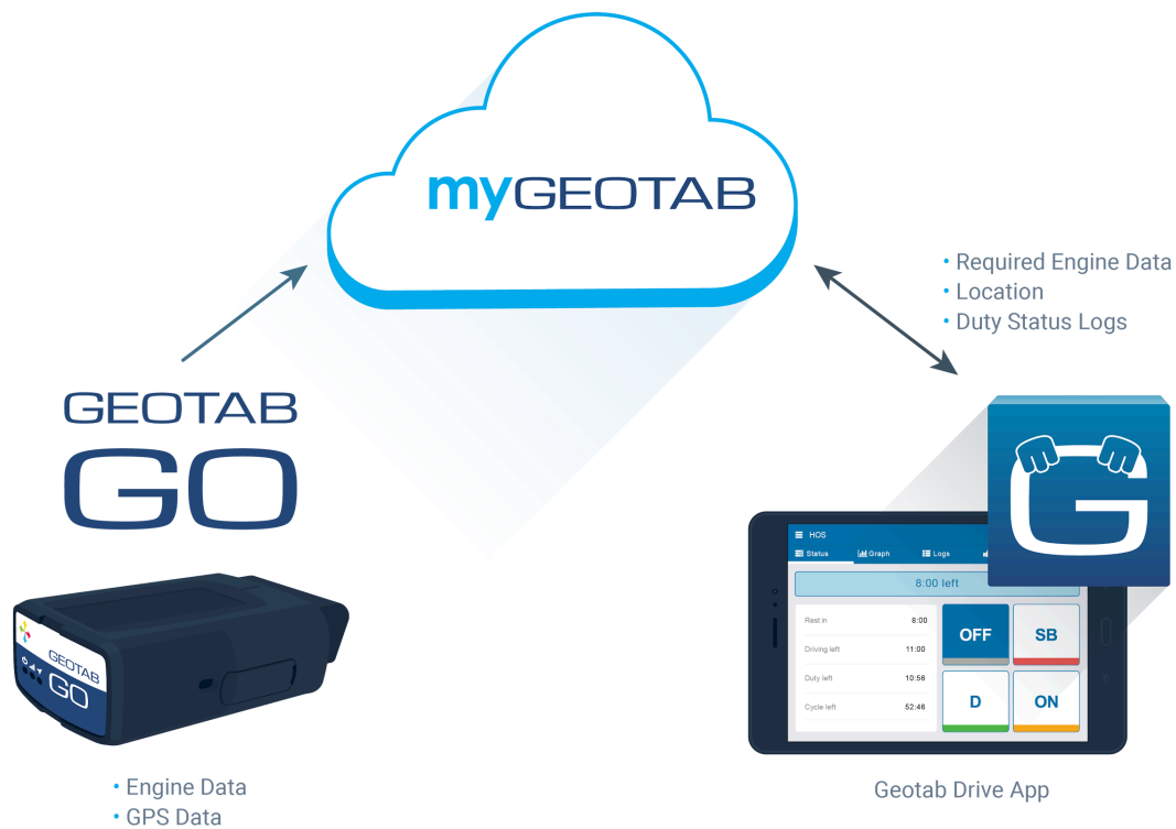
Figure 1: Engine and GPS Data from the GO device is sent to the MyGeotab server. Duty Status logs are created on the server, and then pushed down to the Geotab Drive app together with engine and location information.
