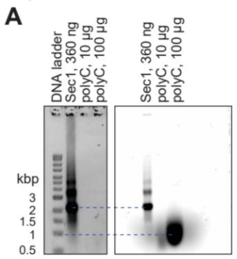
Agarose gel with a DNA ladder. Left shows GelRed; right is Cy3. As you can see, there is a slight laddering effect, but the band appears crisp (few degradation products)
