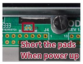
If your unit does not go straight to a red and blue LED, and instead the Blue LED flashes, that means that the unit is booting from the eMMC and jumping the microSD. In order to boot from the
