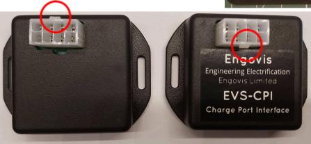
V2 has the connector lock, circled in red on the top. V3 has the connector lock on the bottom.
