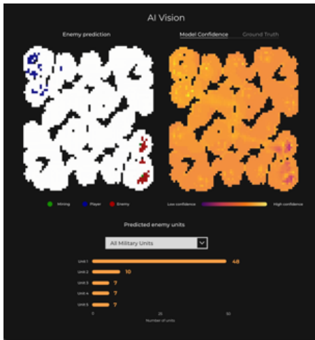
Figure 7. Screenshot of the UI showing opponent's units through the fog of war as predicted by the defogger model, prediction confidence levels, and total predicted unit counts across the map.
