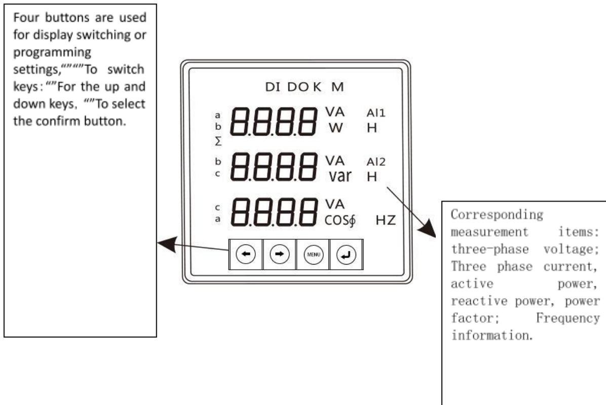
▲The schematic diagram of the display interface takes IED as an example (the page is subject to actual factory production)
