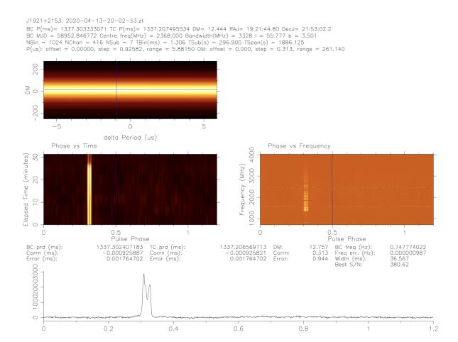
There is no visible sign of phase drift between these two epochs. This can also be verified using pat; e.g. the latter observation has a better S/N, so choose it as the template and run
