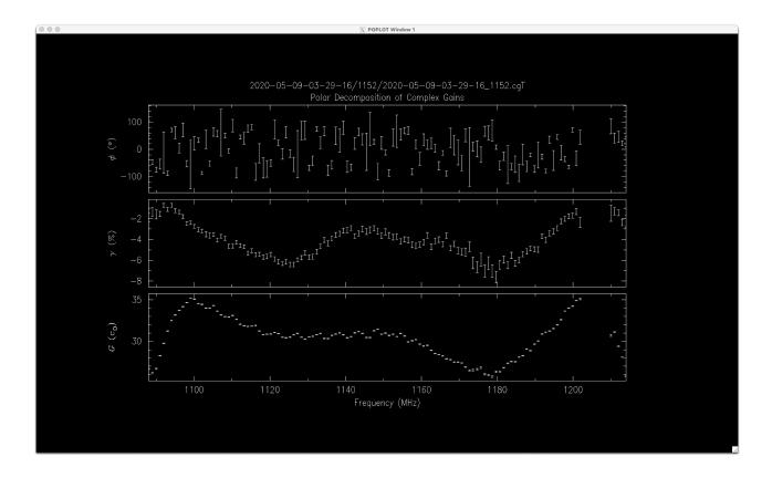
The dropped packet issue can also be seen by zero Stokes U and V in the noise diode observations; e.g. in plots of phase vs frequency
