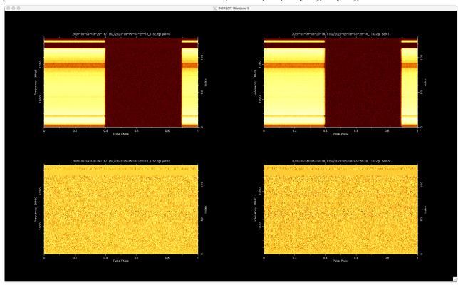
It's also good to plot the phase-versus-frequency intensity of the folded pulsar observations to ensure that there is no residual/missed RFI.
