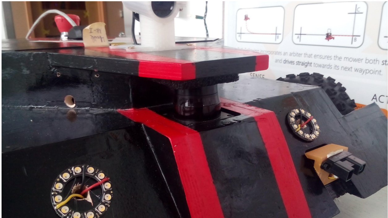
Fig. 21. LIDAR is horizontal, and not on a tilt system.
