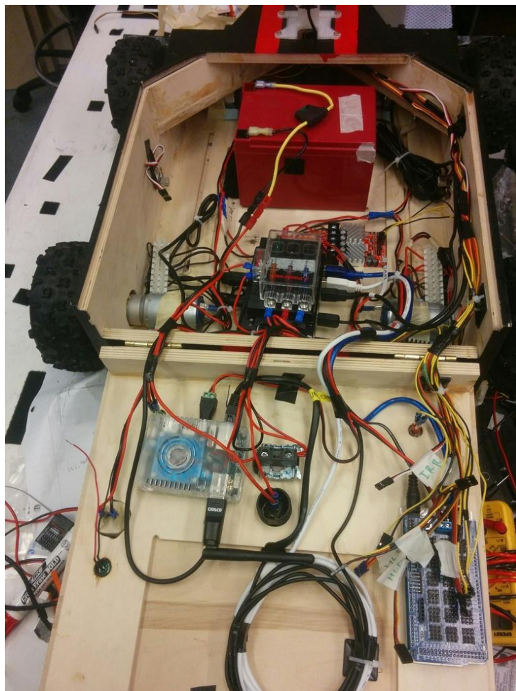
Figure 3: The electrical layout of our robot.
