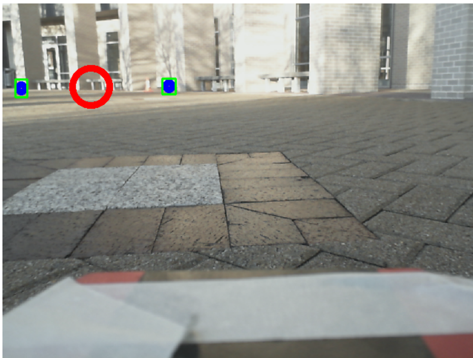
Fig. 20. Cone detection finds the center between cones.
