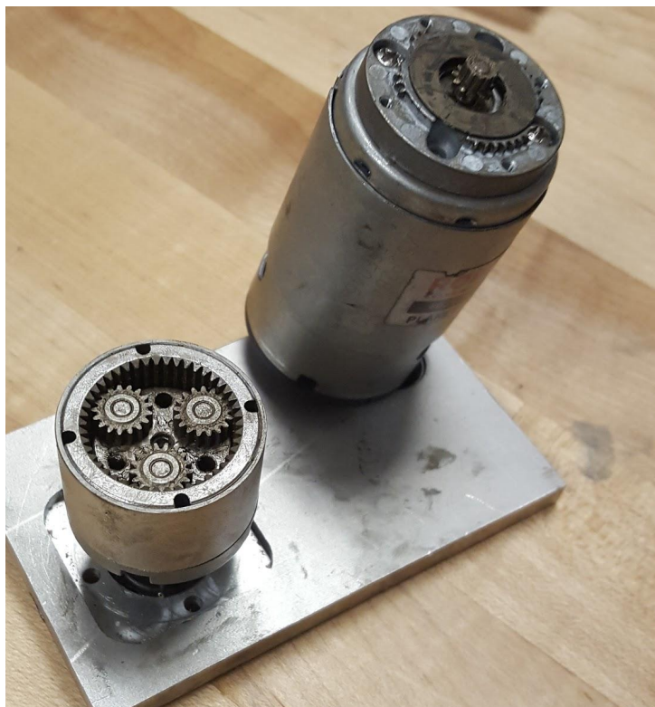
Fig. 18. The sun gear on the motor is sheared off.
