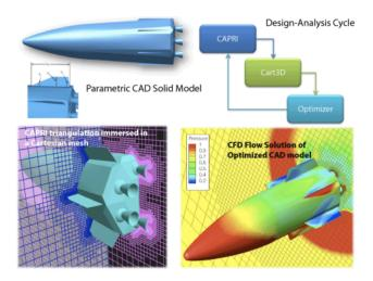
NASA uses parametric modeling in many ways. From communication systems and satellite development, to fluid systems for propellant and spacecraft designs, parametric modeling plays an important role in aerospace designs. Algorithmic models provide fast solutions, and NASA even uses a parametric-based repository for just-in-time problem solving.
