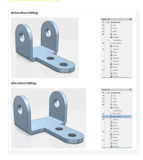
The simple example of the above images shows that one bracket is wider than the other. The push and pull capabilities of direct modeling sets it apart from parametric modeling. The user simply clicks and drags a 3D design feature to manipulate its geometries. Direct modeling fails to account for necessary modifications to the rest of the design or system as a result of the change.
