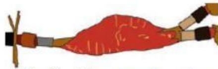
Fig. 8 Wires taped together
