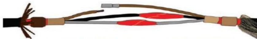
Fig. 7 Taped, crimped connectors on individual cables
