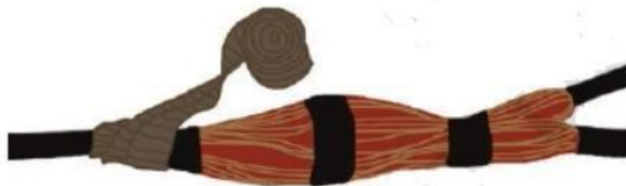
Fig. 9 Wrapping the cable with mesh tape
