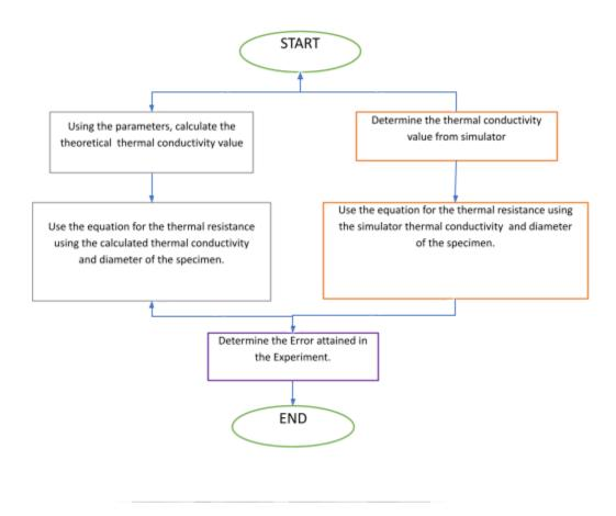
**Objective 3:** Compare the obtained experiment values to the calculated simulator values.
