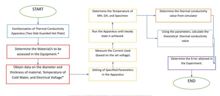
**Objective 2:** Determine the thermal resistance of the sample.
