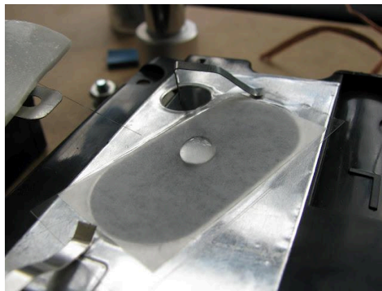
The water sitting on the wax paper, which sits on the glass cover slide, which sits over the speaker, mechanically connected to the membrane through a small piece of PCL
