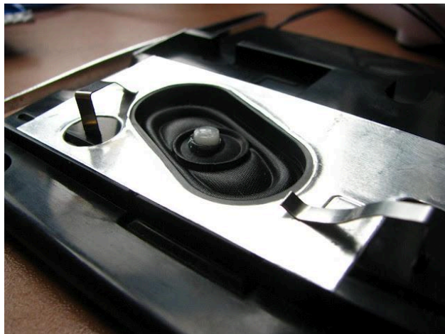
The speaker with the PLC glued on its membrane
