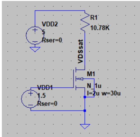
Here is how I calculated R1 = 10.77K in this schematic:
