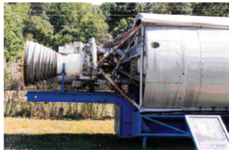
Actual The Engine and Thrust Structure of a Titan Rocket
