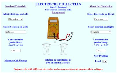
Choose the metal on the left, the anode (black) as Zinc with a 1.00 M solution of Zinc nitrate. Choose the metal on the right, the cathode (red) as copper and the solution concentration of 2.00 M of a copper (II) nitrate solution. Click the "Measure Cell Voltage" to determine the voltage of the system. Change the concentration of the copper(II) nitrate solution and "measure cell voltage" for each of the different concentrations.
