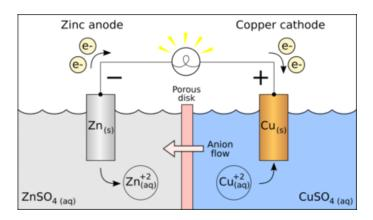
Figure 1. Galvanic cell (or battery) based on the redox reaction.
