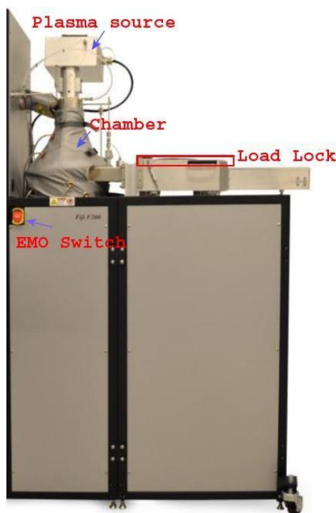
Fig 1. Main items of the Fiji ALD system.
