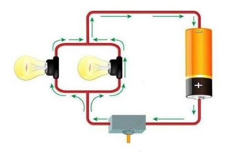
Each load is provided with its own path to the source of supply.
