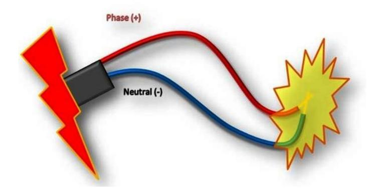
A short circuit may also occur if the insulation between the two cores of the cable are defective. This results in a lower resistance. This causes a large current to flow which can become a hazard.
