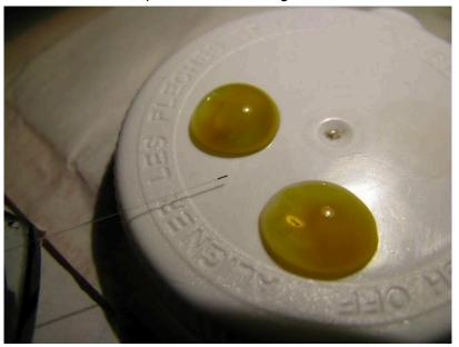
100 um diameter glass fiber after coating in 2 steps. The two drops are the 2 coating environments.
