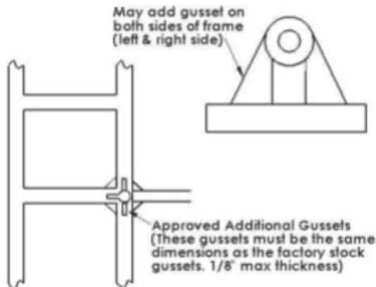
Rear End Housing Upper Link & Rear Trailing Arm Pickup Point
