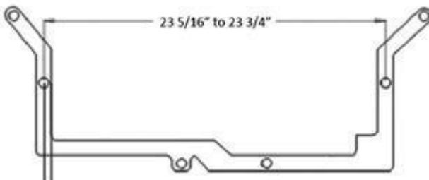
**65. SPINDLES:** The Aluminum spindles (and the spindle pick-up points) must remain Stock, within the Stock dimensions, thickness, location, and configurations. Repairing a broken or cracked aluminum spindle is not permitted.
