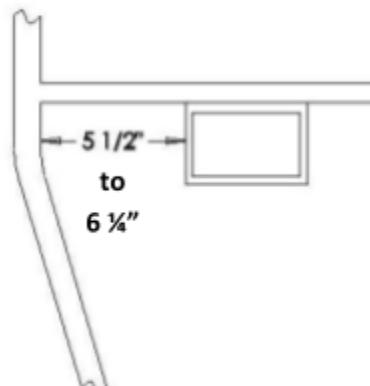
*Note: The measurement for the battery box offset will be taken at the point closest to the crossmember, from the inside of the framemail to the outside of the battery box.*
