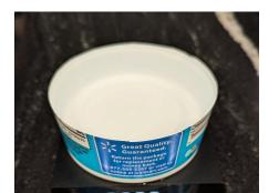
Empty and dry this container as it will now become your "bean density bucket". Set the container on a scale and fill it to the top with green beans, using your finger to smooth and level them. Note the weight of the beans it took to fill the same volume as 250ml of water, then do this calculation to get bean density:
