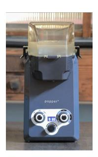
add/subtract time from the timer. Once the timer reaches 3 minutes, the machine automatically kicks into cooling mode to bring the bean temperature down and stop them from roasting further.
